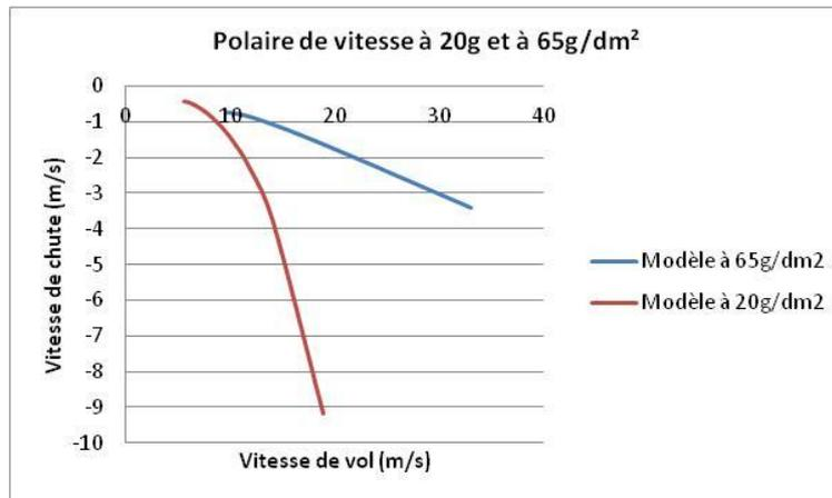
A very light plane could not fly at a speed of 10m/s without sinking drastically (over 2m/s). A heavy plane could go over 20m/s for the same sinking rate.
