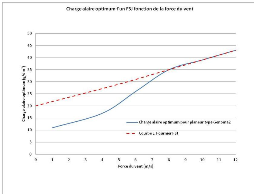
For a wind lower than 5m/s, a F5J plane that is launched inside the lift should be at a wing load lower than 20g/dm<sup>2</sup>. Plane should then be “as light as possible”. I do not believe that a 4m wing span plane can be lighter than 11g/dm<sup>2</sup>. 15 to 17g/dm<sup>2</sup> is still very difficult to obtain for a F5J plane. That’s why I limit the curve to this “still unrealistic” F5J wing load. But who knows...
