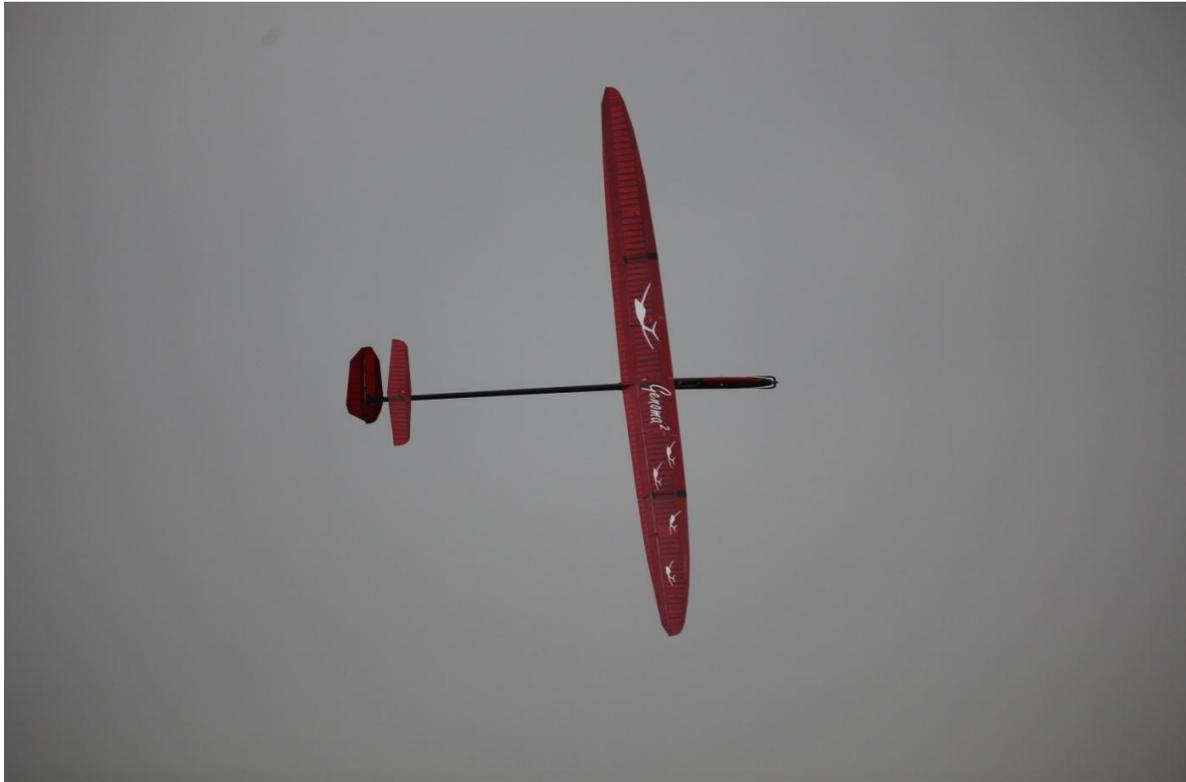
*The Genoma<sup>2</sup> was created for F5J. This plane empty weight could be from 17g/dm<sup>2</sup> to 45 g/dm<sup>2</sup>. During the 2 of the 3 F5J local contests made during a year, the plane finished at the third and at the second place. Don't think the pilot is good! The plane is better.*
