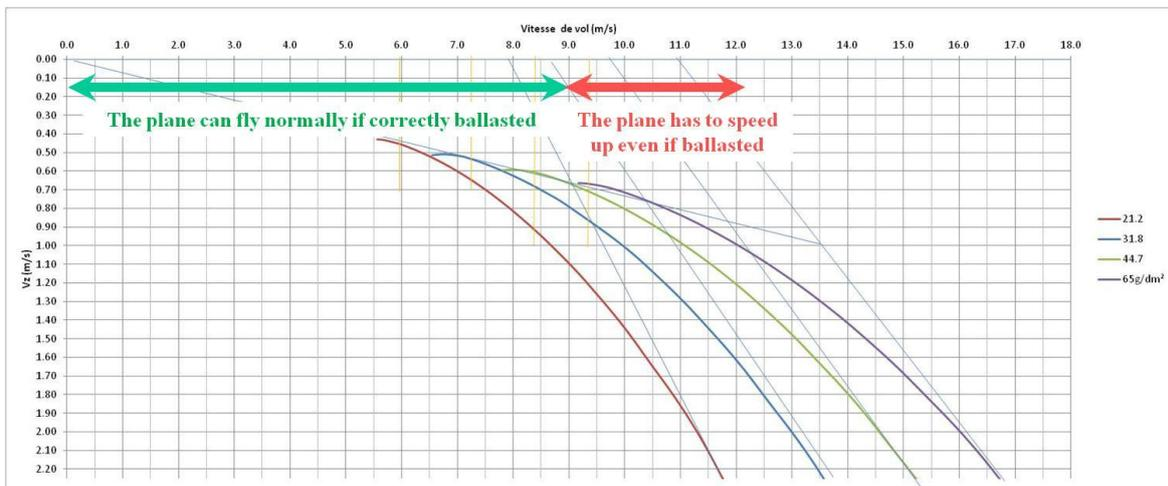
**Up to 9m/s wind, a plane can be ballasted as per FAI regulation and flew in a standard way. It is possible to fly at minimum sinking rate... Over 9m/s, this is no more true, and even if fully ballasted (at 75g/dm<sup>2</sup> as allowed), the plane has to speed up to go upwind. This then requires a specific trimming (pitching) for such occasion.**
