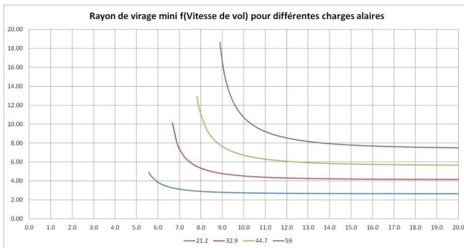
***Circling radius for a defined flying speed when circling. All is expressed for different wing load.***
