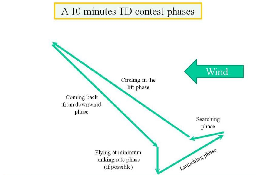
**To succeed a TD flight, plane need to reach altitude, find a thermal, take it for as long as required to finish a 10 min flight, return home for landing with an altitude margin. For high wind, this requires to go very far downwind (up to 2 km) and reach a very high altitude (6 to 700m).**
