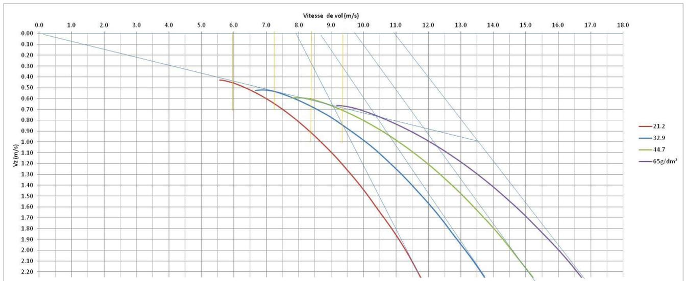
**Sinking rate =  $f(\text{speed})$  of the Genoma<sup>2</sup> plane for different wing load. If you know a polar for one wing load, you can deduct the others ones for any wing load by changing it in the speed and sinking rate formulas. The error made by not taking into account the Reynolds variation effect will not be so important.**
