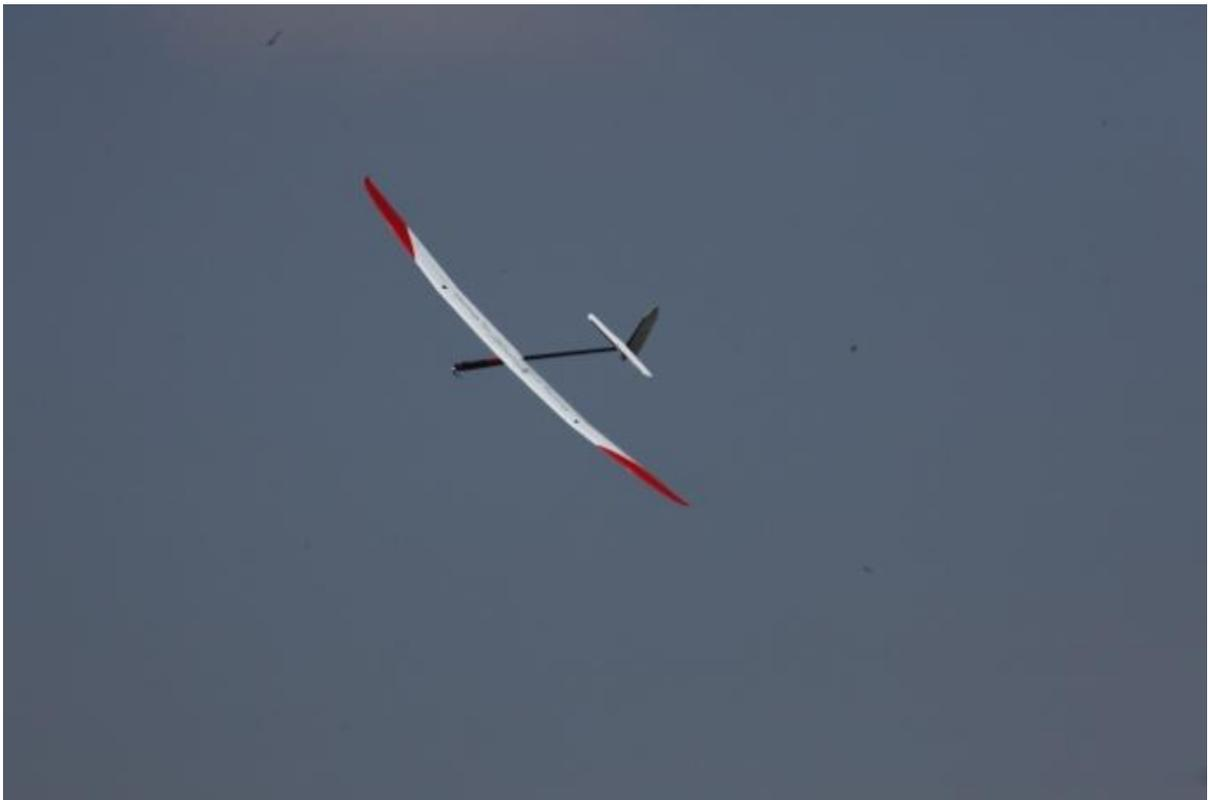
*A way to transform a F3J plane into a F5J one: Take a standard 4m F3J wing (here a Xplorer 4000) and install it on a Genoma<sup>2</sup> fuselage. This works pretty well specially for the circling ability. Of course, the minimum wing load is increased.*
